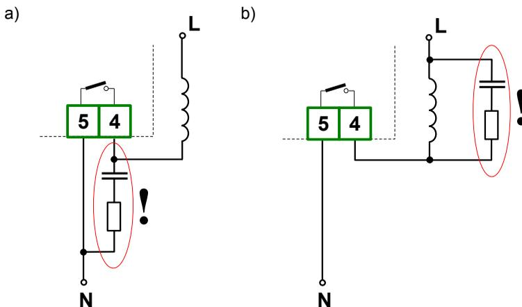
Figure 4.9. Examples of suppression circuit connection:
