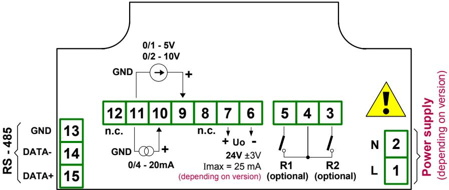
Figure 4.3. Terminals description (relay outputs)
