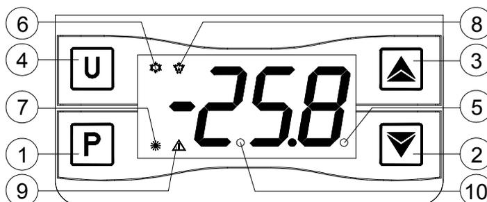
**1 - Key P** : Used for setting the Set point (press and release) and for programming the function parameters (hold pressed for 5 sec.) In programming mode is used to enter in parameters edit mode and confirm the values.
