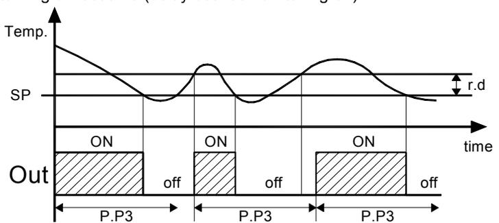
During the output inhibition the led OUT (Cool o Heat) blinking. It is also possible to prevent activation of the output after the instrument is turned on, for the time set in the parameter "P.od". During the power on delay phase, the display shows the indication od, alternating with the normal visualisation. All the functions are disabled by relative parameters = oF.
